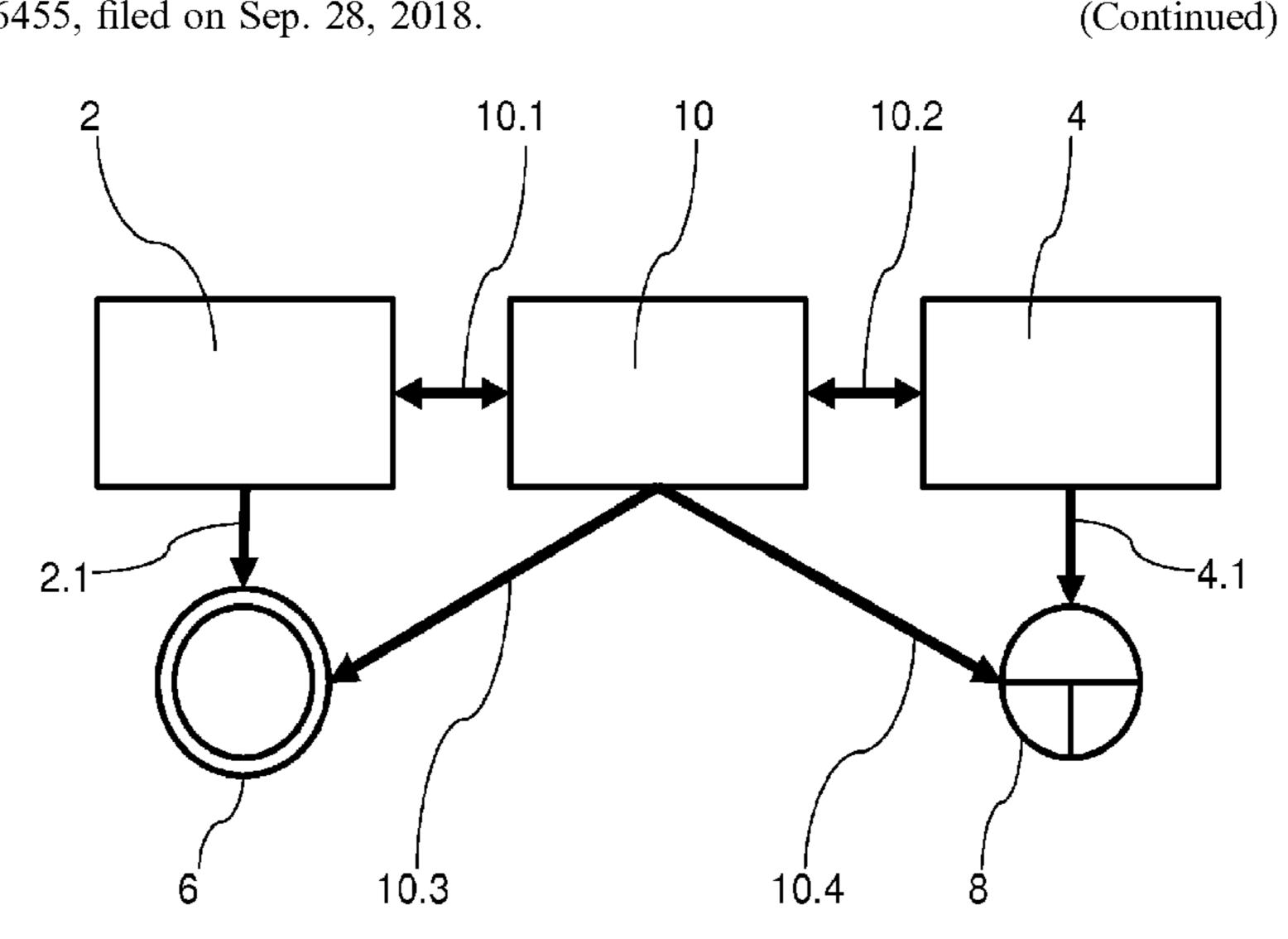
control system has a third control unit for controlling the first function and the second function of the motor vehicle and, depending on the receipt of a fault signal of the first and/or second control unit by the third control unit, the third control unit can be configured such that the motor vehicle first and/or second function corresponding to the faulty control unit can be controlled by means of the third control unit alone.
