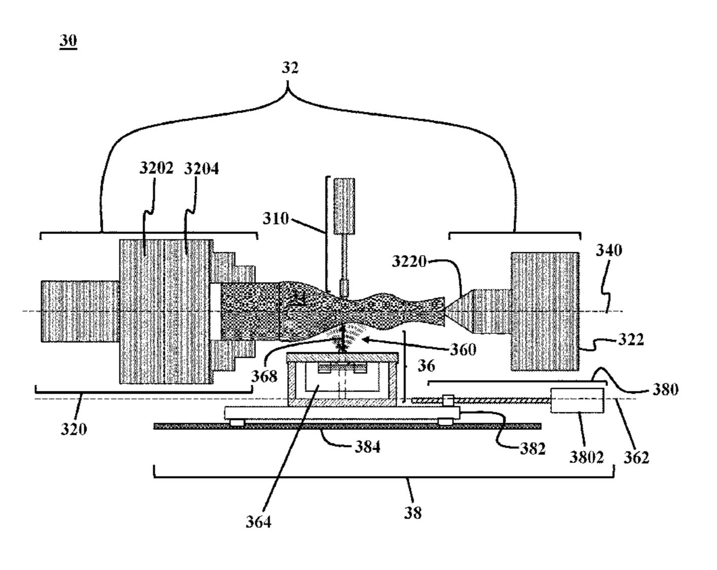
magnetic field and the outer surface of the workpiece along a first axis perpendicular to the longitudinal axis of the workpiece. The system may further include a control unit that may be coupled to the magnetic abrasive brush and may be configured to adjust a magnetic flux density of the magnetic field based on the measured working gap at any given instant.
