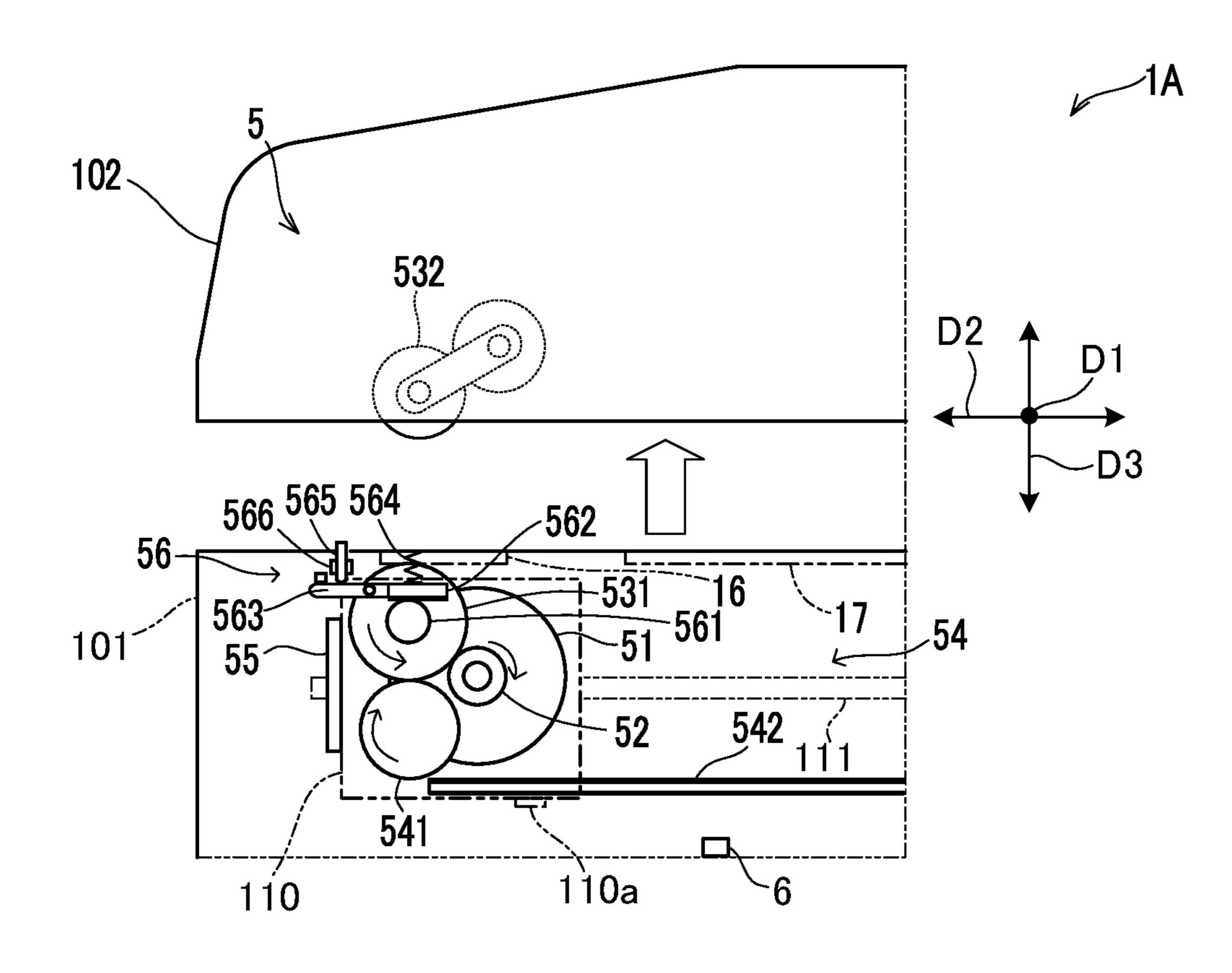
IMAGE READING DEVICE AND IMAGE FORMING DEVICE COMPRISING A DRIVE DEVICE CONFIGURED TO SELECTIVELY APPLY A DRIVING FORCE TO THE CARRIAGE AND THE PLUTALITY OF PAIRS OF CONVEYANCE ROLLERS, WHEREIN THE DEVICE DRIVER INCLUDES AN ABUTTING MEMBER, A MOTOR, A CARRIAGE THAT ROTATES IN CONJUNCTION WITH THE MOTOR SUPPORTS A FIRST MAIN BODY GEAR TO MESH WITH A COVER INPUT GEAR AND A SECOND MAIN BODY GEAR TO MESH WITH A MAIN RACK GEAR
