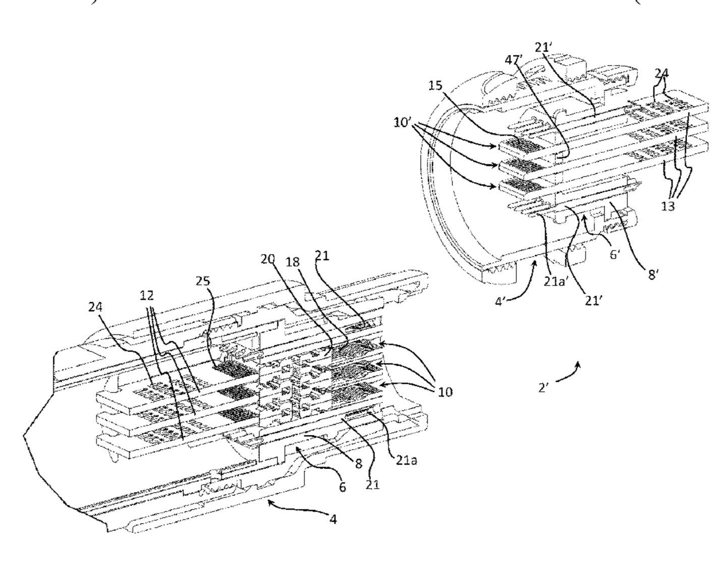
module housing, the terminal modules having a width W to height H ratio W/H greater than three.
