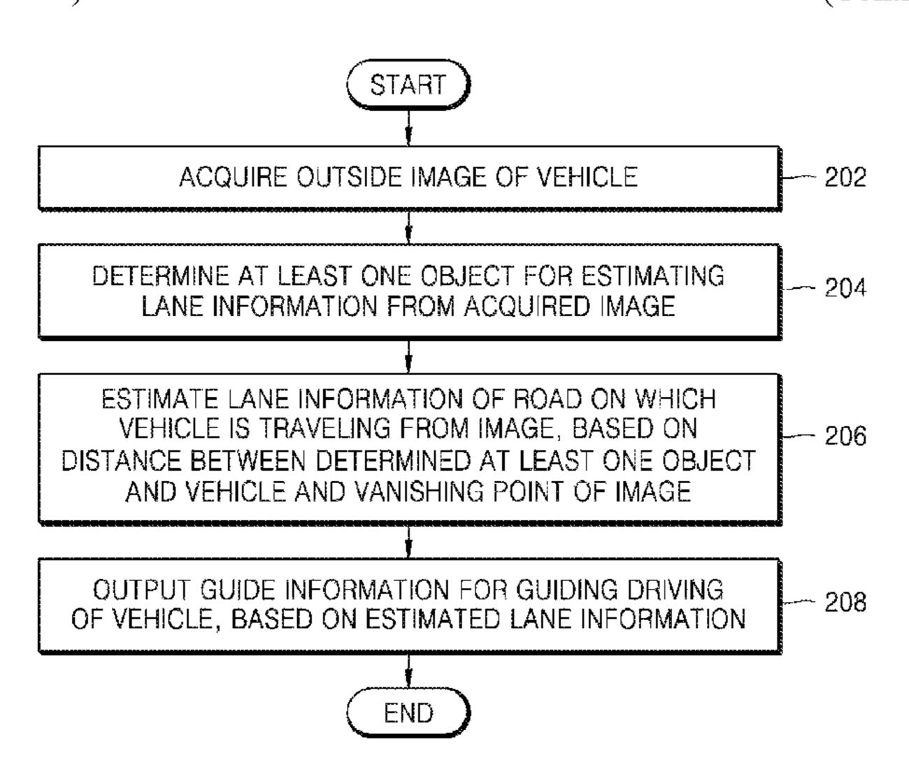
instructions to: determine, from the captured image, at least one object for estimating lane information; estimate, from the image, lane information of a road on which the vehicle is traveling, based on a distance between the determined at least one object and the vehicle and a vanishing point of the image; and output guide information for guiding driving of the vehicle based on the estimated lane information.
