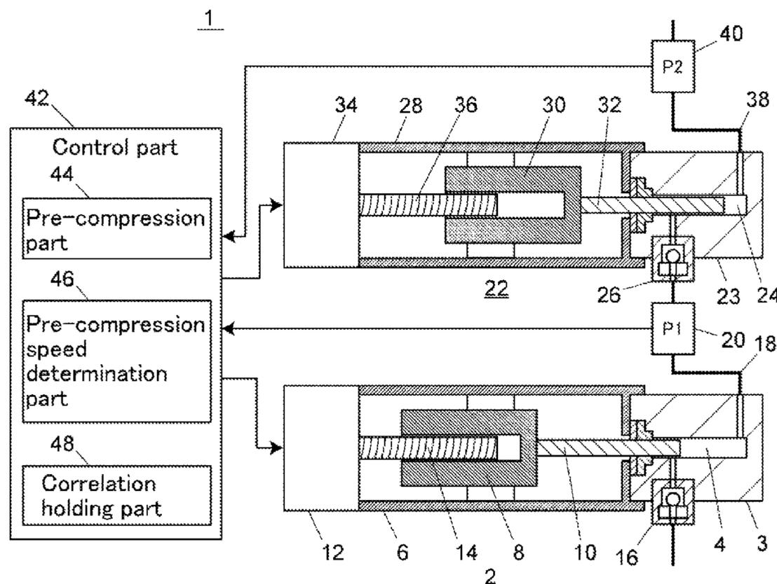
chamber is completed and during the non-discharge time to execute a pre-compression process to perform a discharge operation until a non-discharge pressure is substantially the same as a feeding pressure based on output of the feeding pressure sensor and output of the non-discharge pressure sensor. The pre-compression speed determination part determines a pre-compression speed of the closed pump in the pre-compression process.
