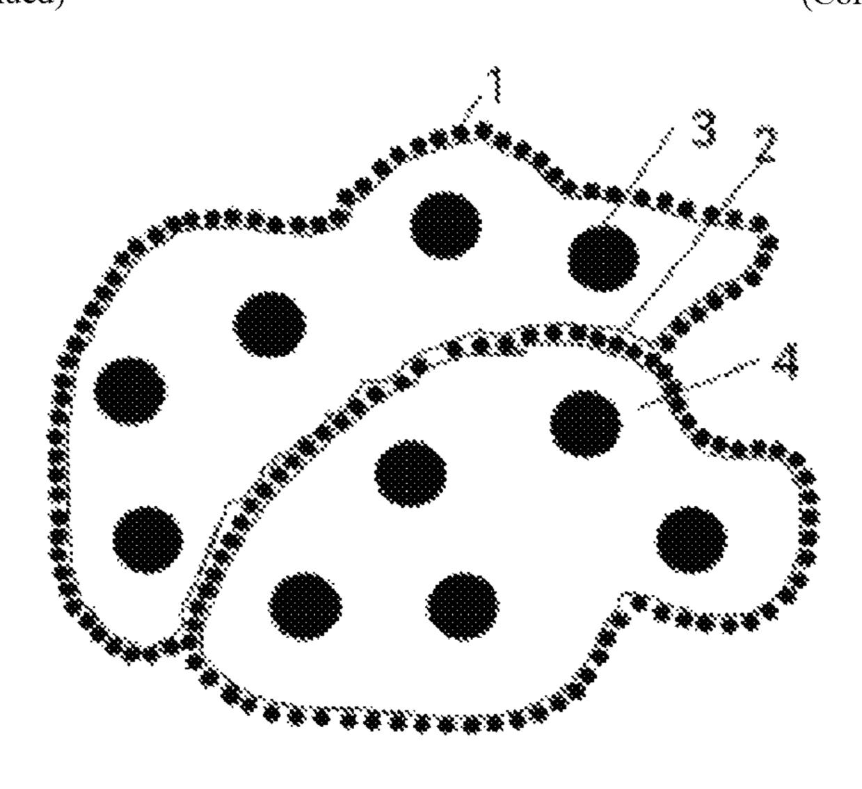
additives may optionally have a diameter of between 0.05 mm and 5 mm, preferably between 1 mm and 3 mm. Advantageously, the additives can be selected from at least one of acetylene coke, fluid coke, flexi coke, shot coke, carbon black, non-graphitisable carbons (chars), non-graphitic anthracite, silicon carbide, titanium carbide, titanium diboride or mixtures thereof.
