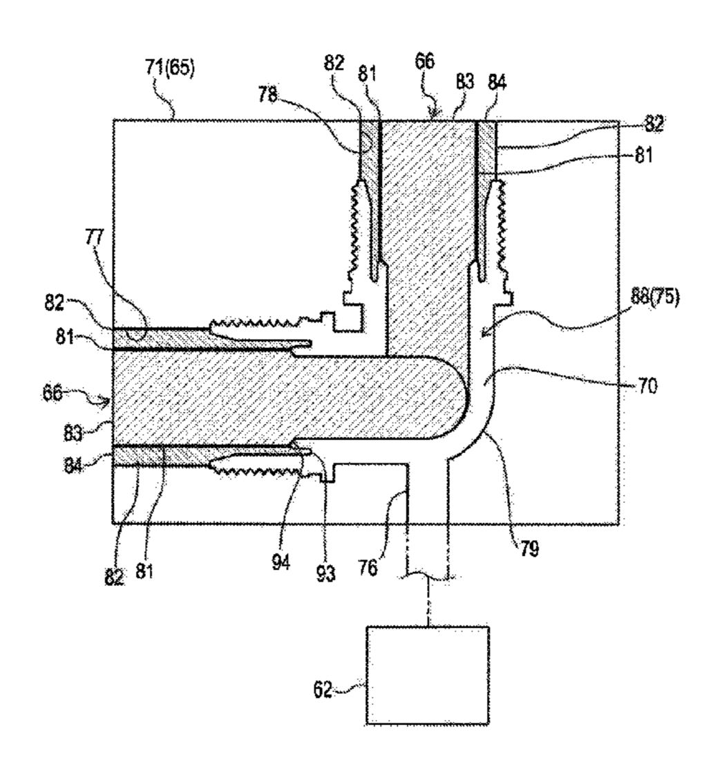
second mold has a gap that connects the cavity to a discharge space outside the cavity and allows gas to flow.
