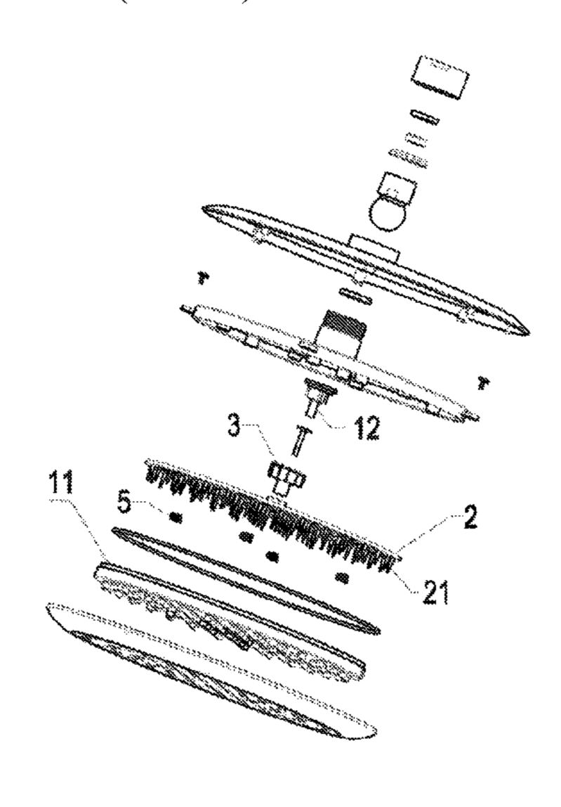
about the axial direction of the deposit removal needle plate in a corresponding one of the plurality of water outlet holes.
