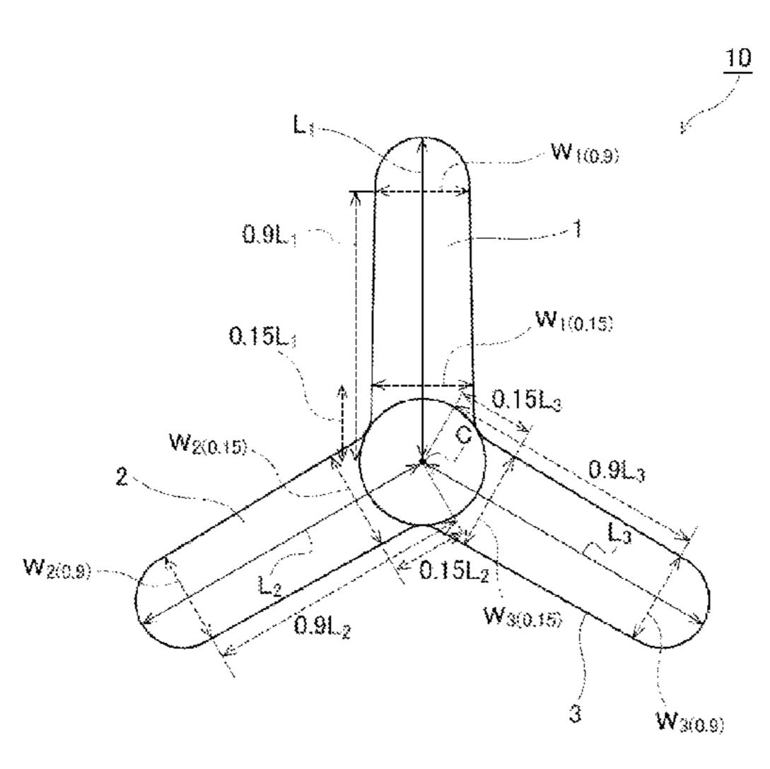
projection, and a third projection and the lengths and widths thereof satisfy predetermined conditions.
