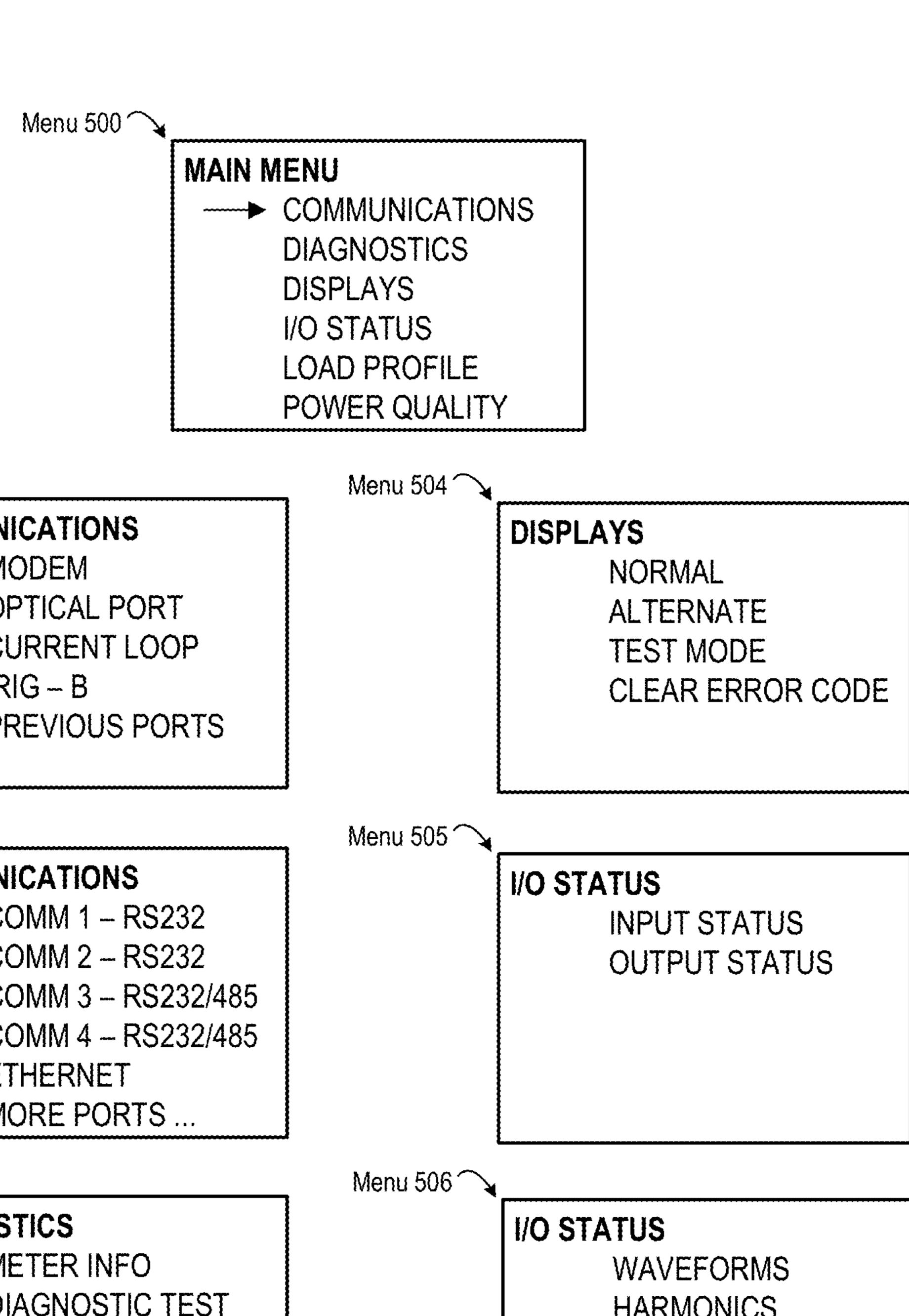
Menu 501 7 COMMUNICATIONS MODEM OPTICAL PORT CURRENT LOOP IRIG - B PREVIOUS PORTS Menu 502 7 COMMUNICATIONS COMM 1 - RS232 COMM 2 - RS232 COMM 3 - RS232/485 COMM 4 - RS232/485 ETHERNET MORE PORTS ... Menu 503 ^ DIAGNOSTICS METER INFO DIAGNOSTIC TEST HARMONICS VECTOR DIAGRAM SAGS & SWELLS ERROR CODES LCD CONTRAST ACCURACY TEST
