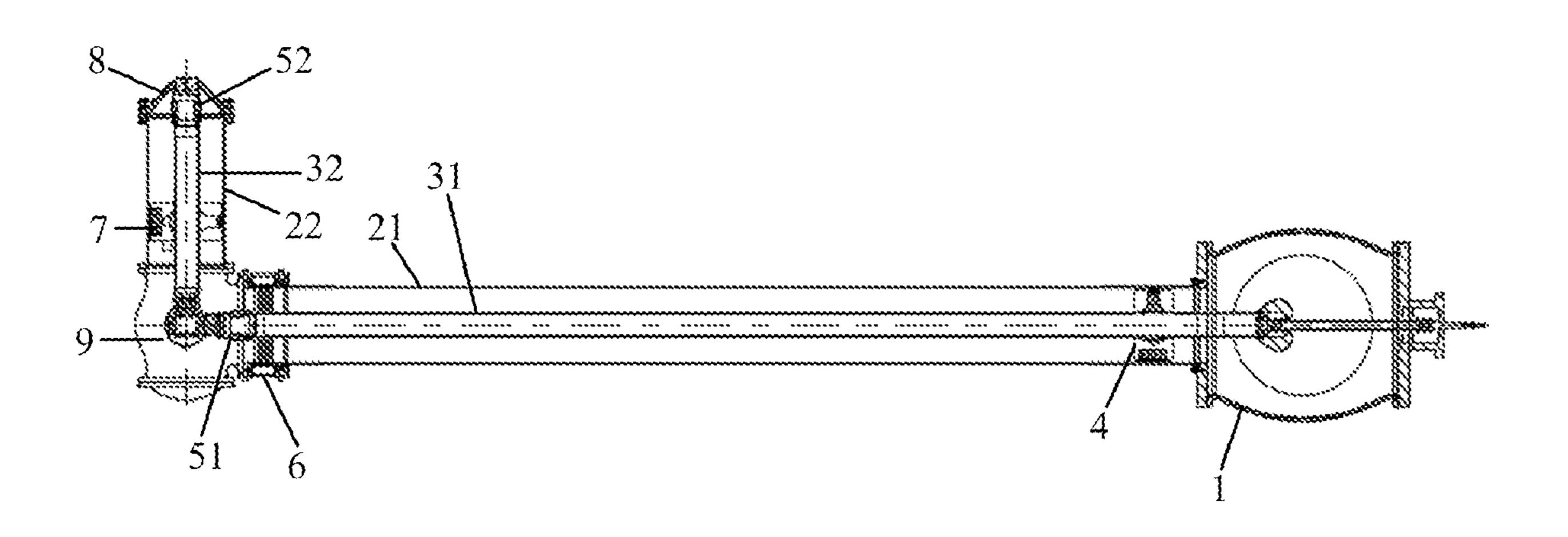
the working condition of the fixed tri-post insulator under abnormal forces when the GIL experience foundation settlement.
