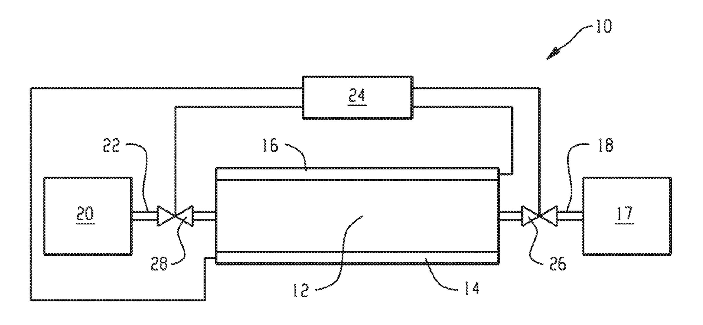
caloric material and a heat sink, and a second thermal flow path between the electrocaloric material and a heat source.
