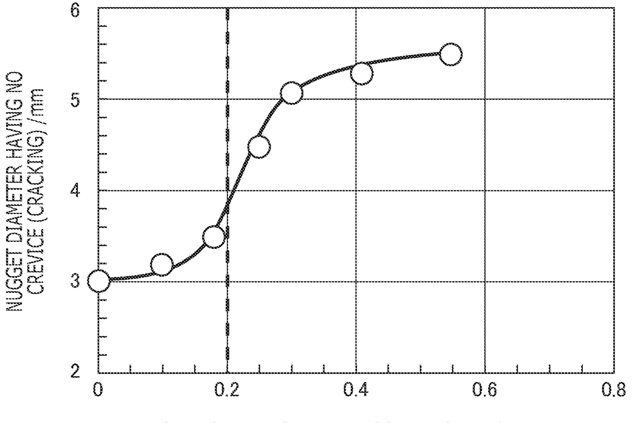
AMOUNT OF DIFFUSIBLE HYDROGEN IN STEEL /mass.ppm
