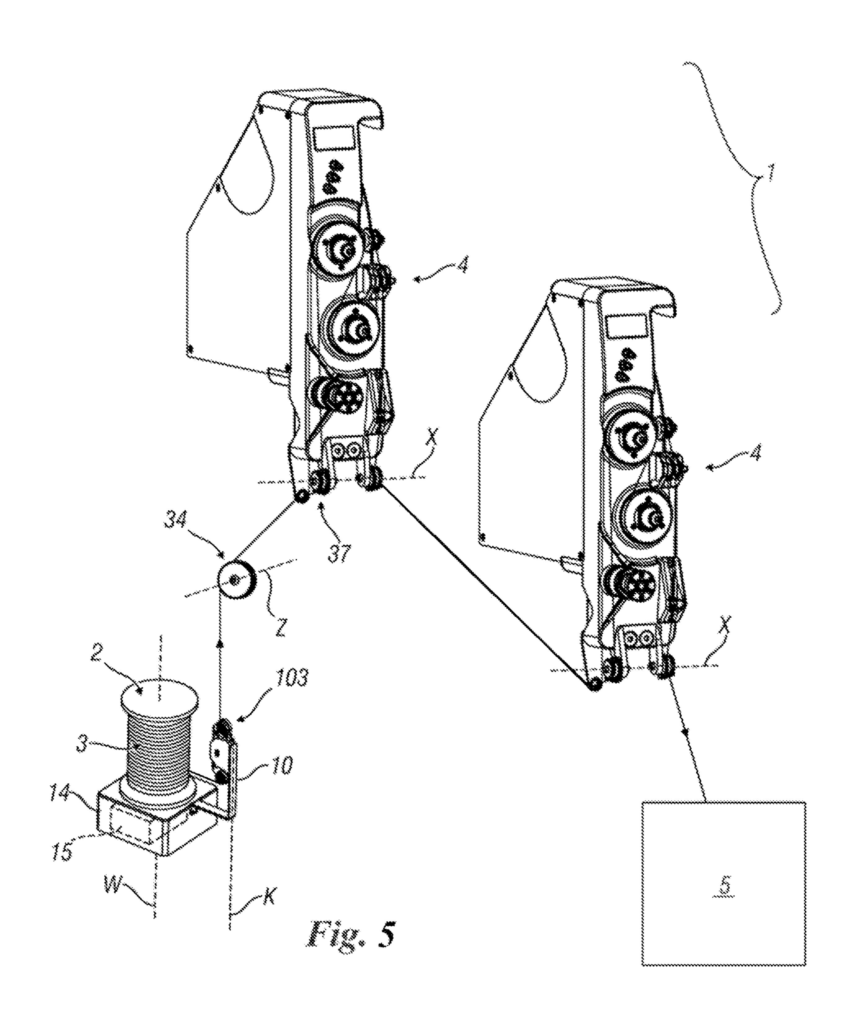
METHOD AND SYSTEM FOR FEEDING A TWISTED BRAIDED METAL CABLE OR FLAT WIRE FROM A CORRESPONDING SUPPORT WITHOUT ALTERING THE STRUCTURE OR SHAPE OF THE WIRE
