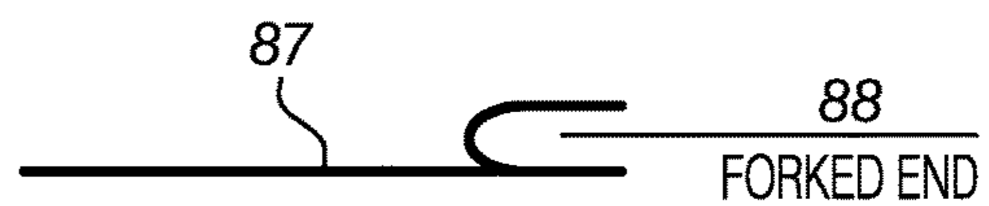
SIDE VIEW OF TWO PRONGED PUSHER 87
