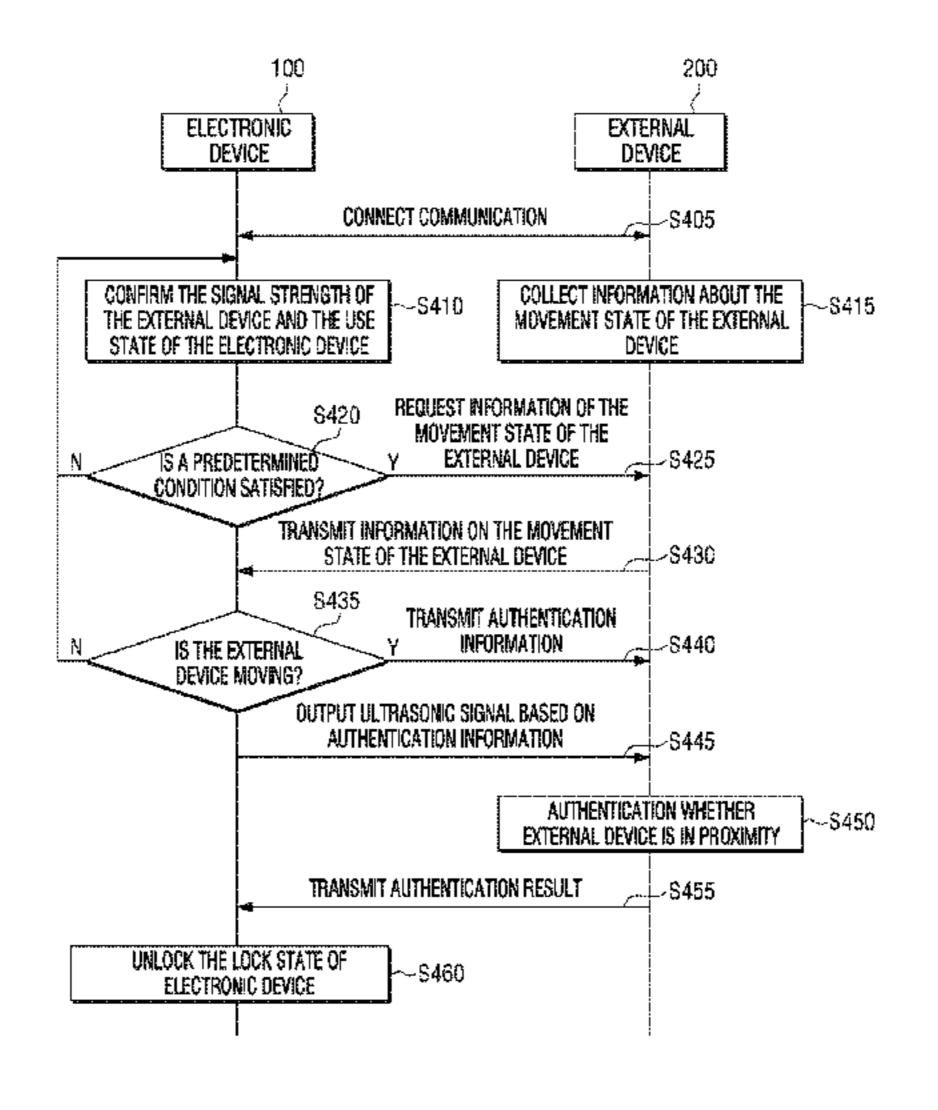
the authentication information, and an authentication result in response to the ultrasonic signal may be received from the external device.
