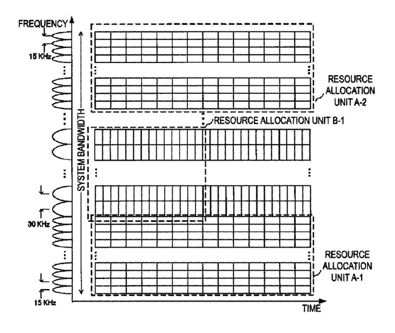
transmitter generates the OFDM signal by using a plurality of the subcarrier spacings, and the transmitter configures a transmit power of the uplink data channel, based on the subcarrier spacing of subcarriers to which the uplink data channel has been mapped.
