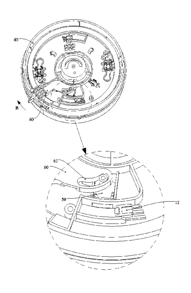
the gripping slots. The module is switchable between the first position and the second position.
