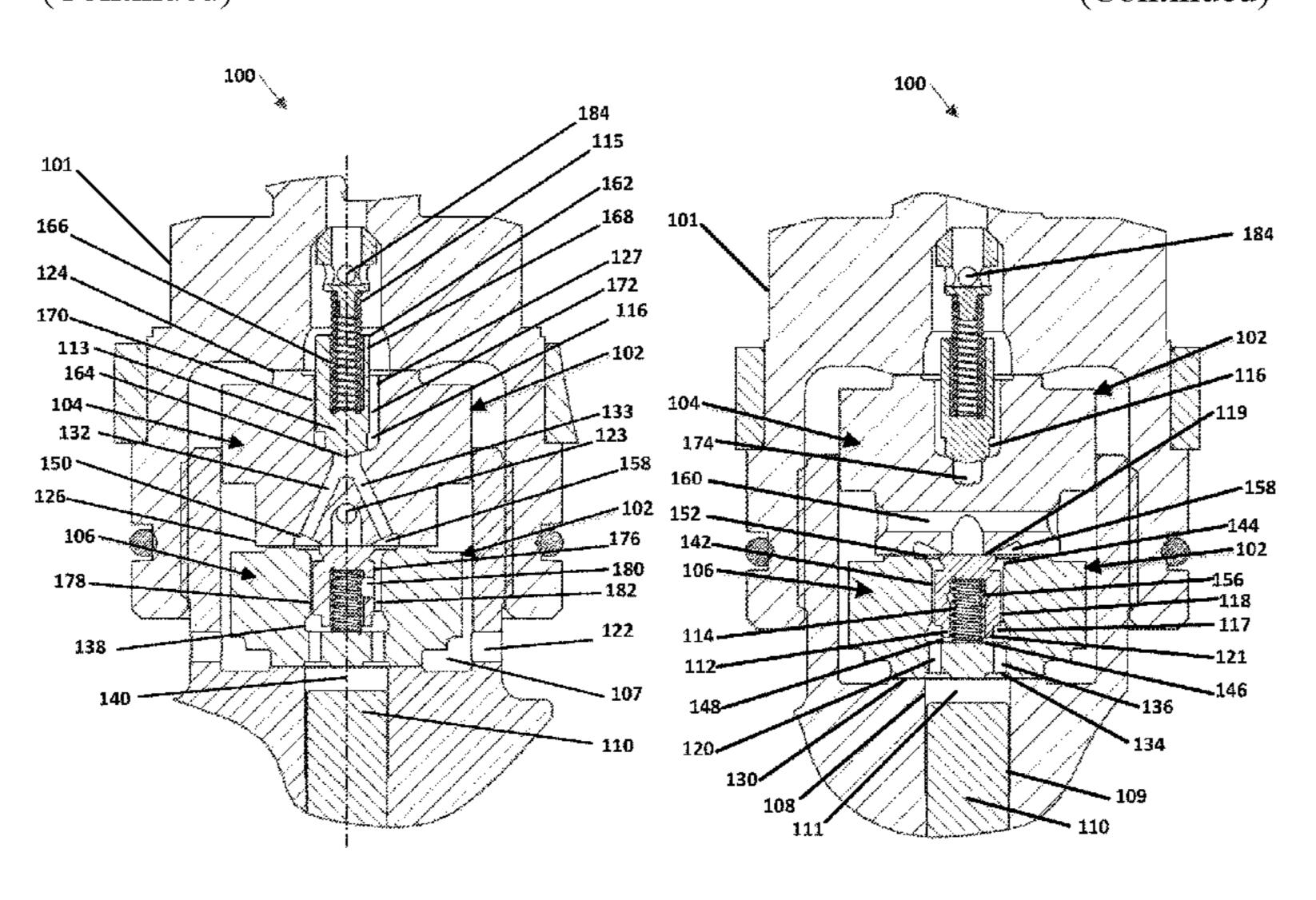
pumping chamber, the second insert including a central bore in flow communication with a fuel inlet, a plurality of through holes in flow communication with the pumping chamber.
