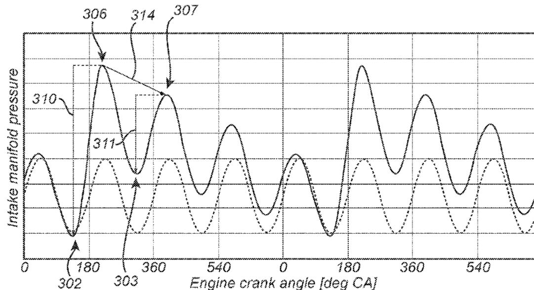
..... Intake manifold pressure - fault free system
