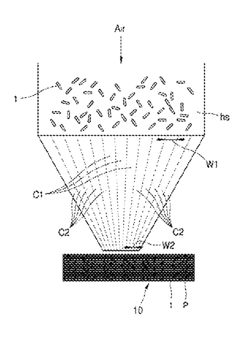
ment composite material, and a sandwich structure. The method for preparing a unidirectionally aligned discontinuous fiber reinforcement composite material comprises discontinuously aligning short fibers on a polymer substrate in one direction by using an air-laid method.
