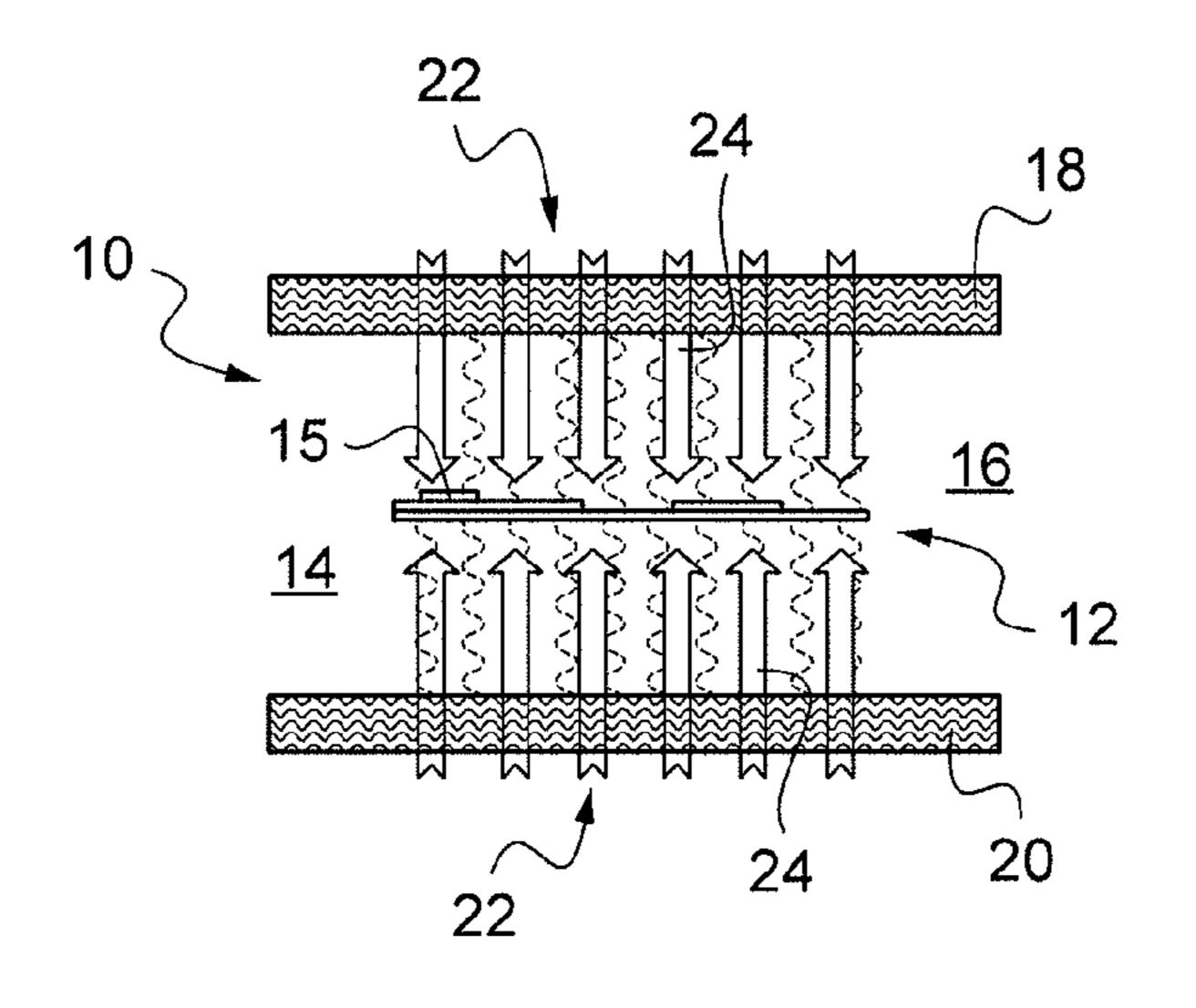
a forming mould. Step b) further involves simultaneously spraying a gaseous fluid onto the surface of the preform in order to preserve the surface.
