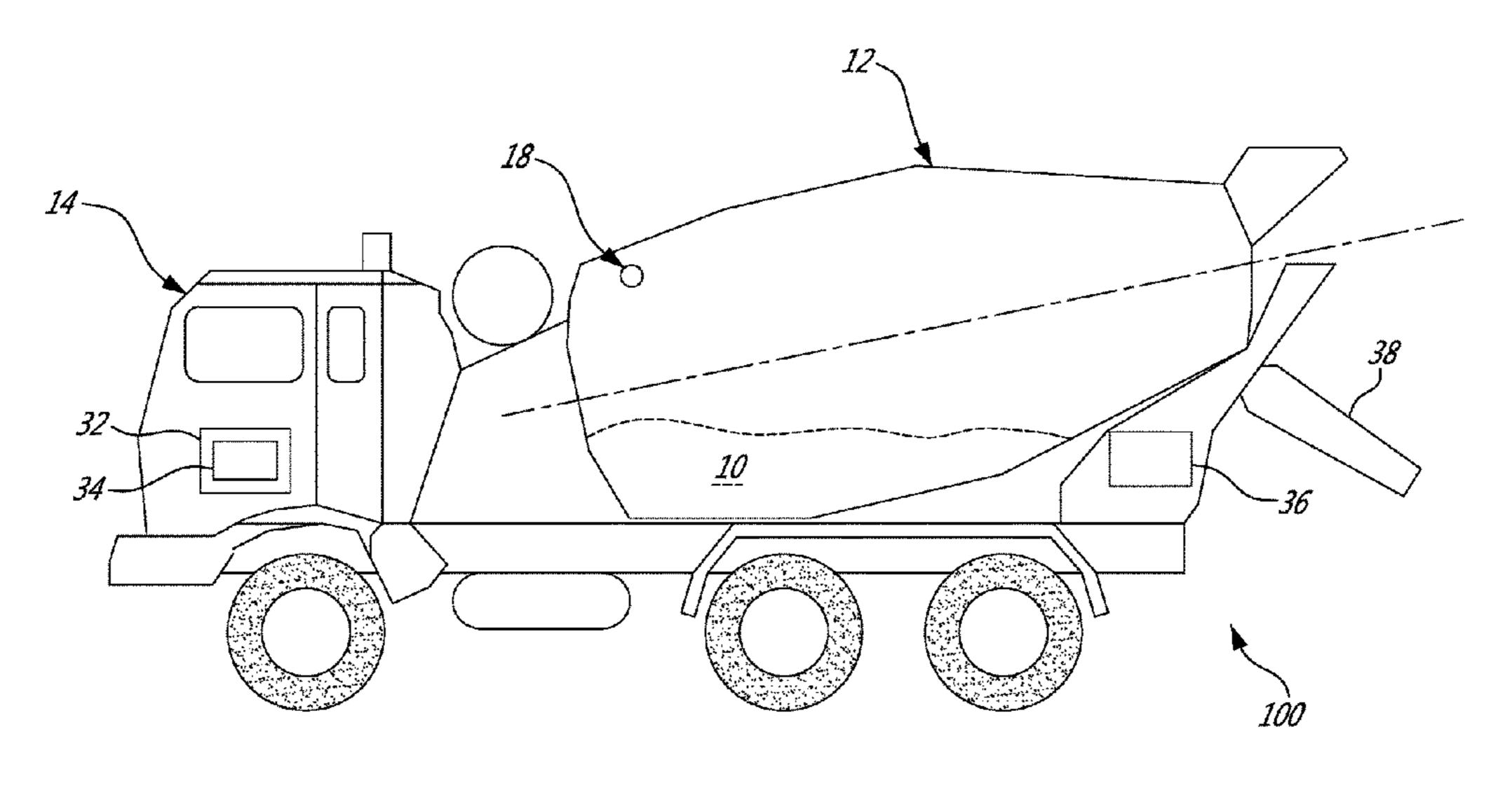
based on the reference workability values associated with reference pressure values corresponding to the received pressure value in the at least two calibration data sets and on the viscosity difference value; and handling the fresh concrete based on the determined workability value.
