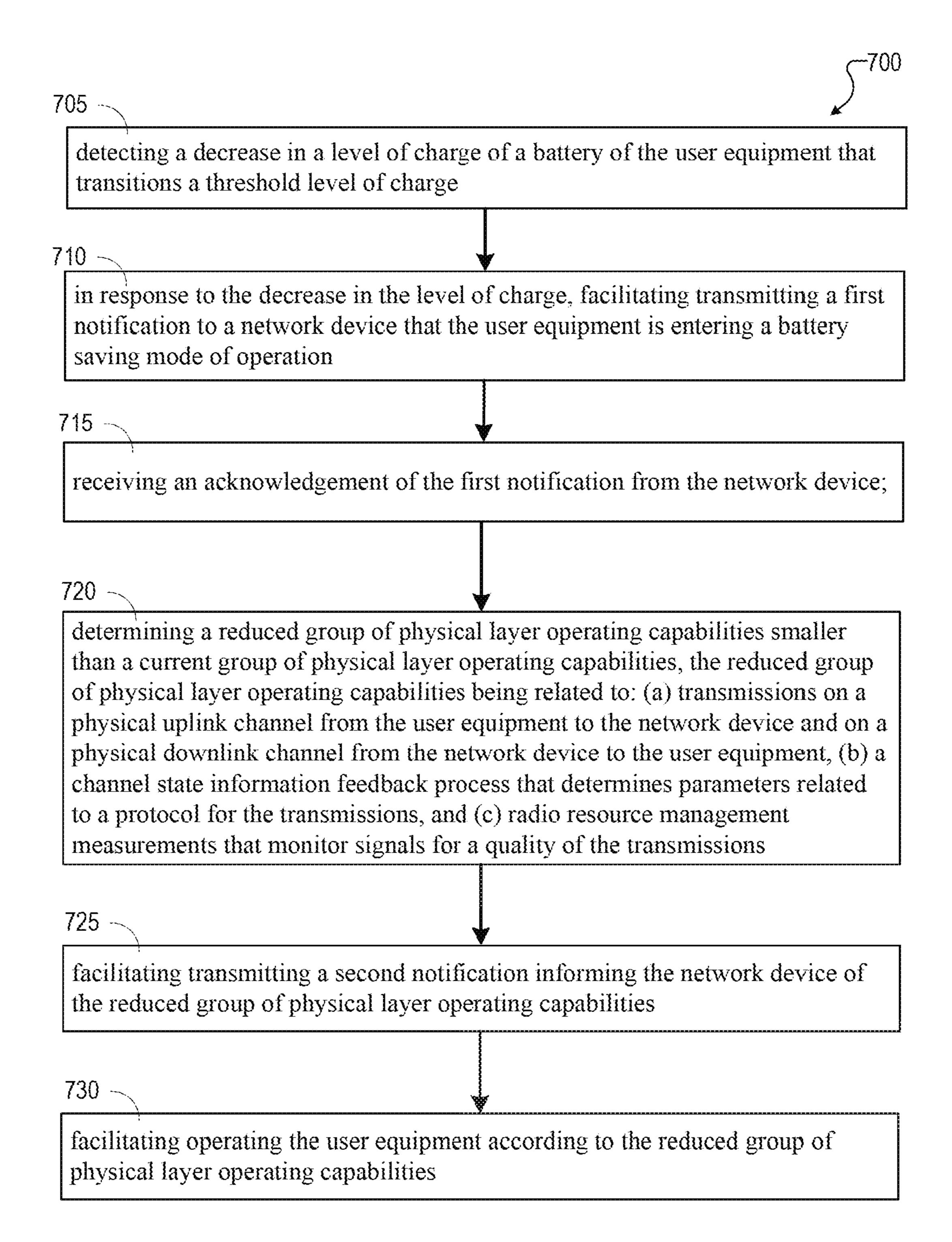
receiving, from a user equipment, a notification that the user equipment is entering a battery saving mode of operation
