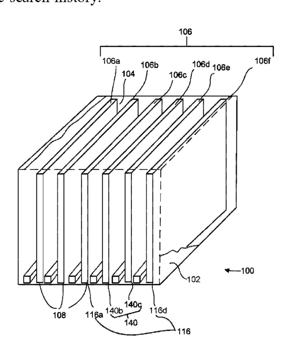
of input switch terminal and a plurality of output switch terminals. Furthermore, each line card and each fabric card comprises a card controller where the card controller selectively couples one or more input switch terminals of a cross-point switch to the output switch terminals of that cross-point switch. The cross-point switches being manipulated by the card controller may belong to one or more different cards within the same video router.
