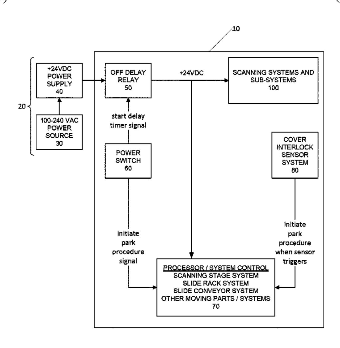
device. This allows the digital pathology device to resume normal operation upon power up.
