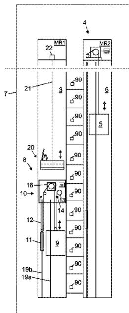
or goods between vertically displaced floors, during which using the method comprises performing construction work in the first hoistway above the traveling zone of the car of the construction time elevator.
