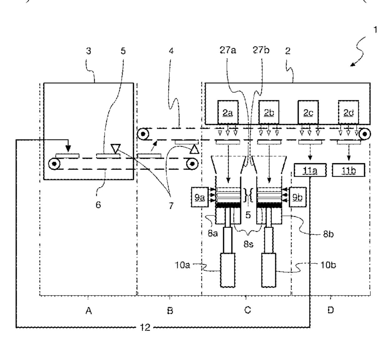
data carriers conveyed along the conveying device from the latter in order to transfer them directly into a card magazine and to stack them therein.
