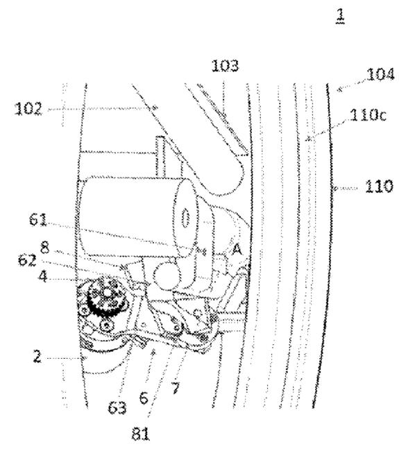
and a transport position in which the pinion (4) is distanced from the tyre (110) and retracted beneath the seat (103).
