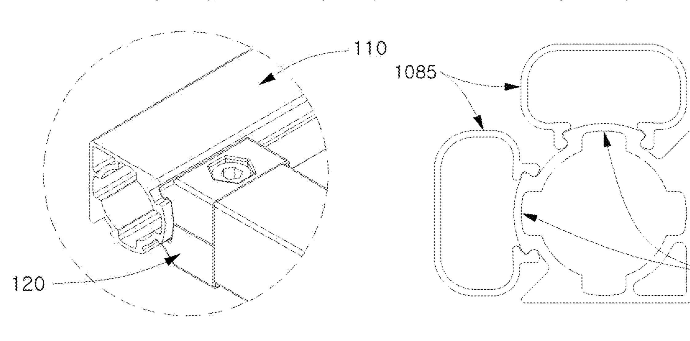
rack pipe can be reinforced relatively more than that of a conventional rack pipe having a curved shape so as to allow the rack pipe to be used as a pillar for supporting heavy materials or receiving a heavy load, thereby enabling stable support.
