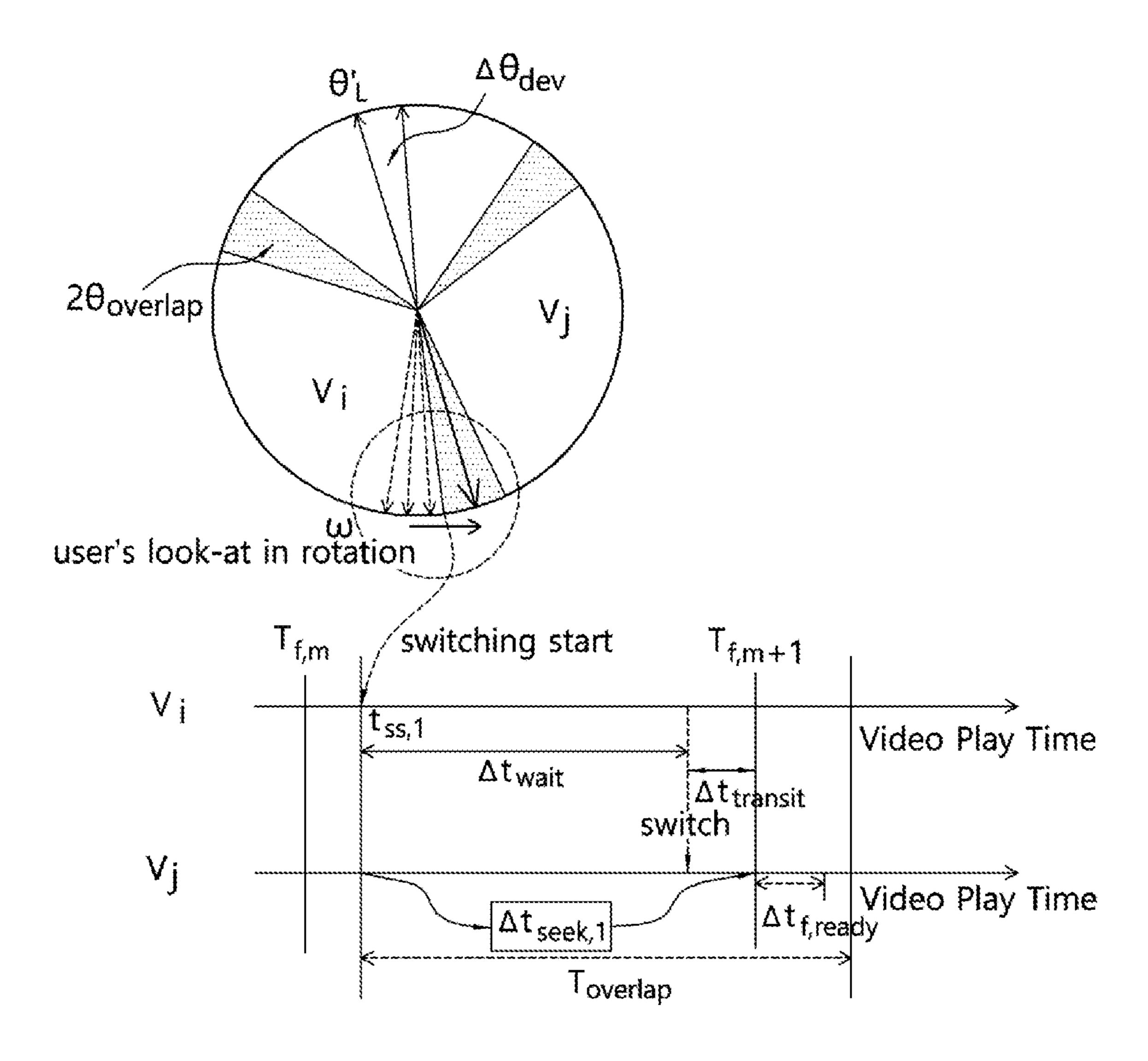
$\Delta t_{seek,1}$ , seek time for key frame of case 1  $t_{ss,1}$ , switching start for key frame of case 1  $\Delta t_{wait}$ ,  $V_i$  run time before switch  $\Delta t_{f,ready}$ ,  $V_j$  subsequent frame ready time  $\Delta t_{transit}$ ,  $V_i - V_j$  frame transit time
