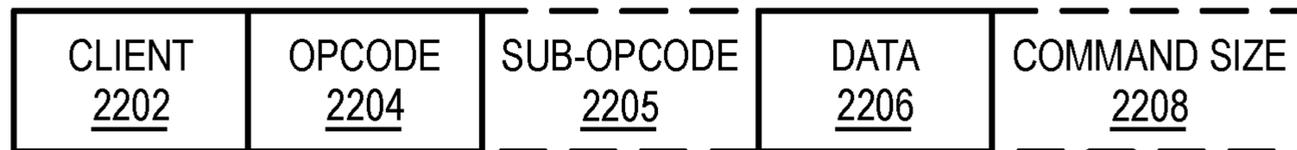
FIG. 22B GRAPHICS PROCESSOR COMMAND SEQUENCE
