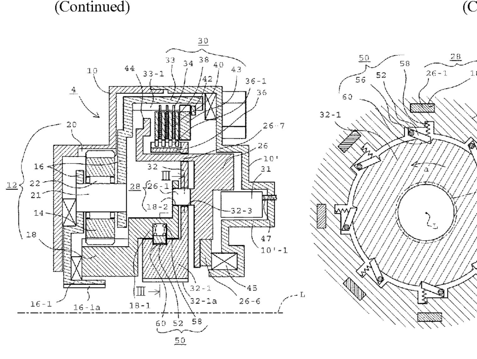
(50) is coincident with that of the dog clutch (28). When shifting from the second speed to the first speed, since the rotational phase of the dog clutch (28) is adjusted by the ratchet-type one-way clutch (50), the shifting is instantaneously completed without waiting operation for the phase adjustment, resulting in preventing a transmission shock.
