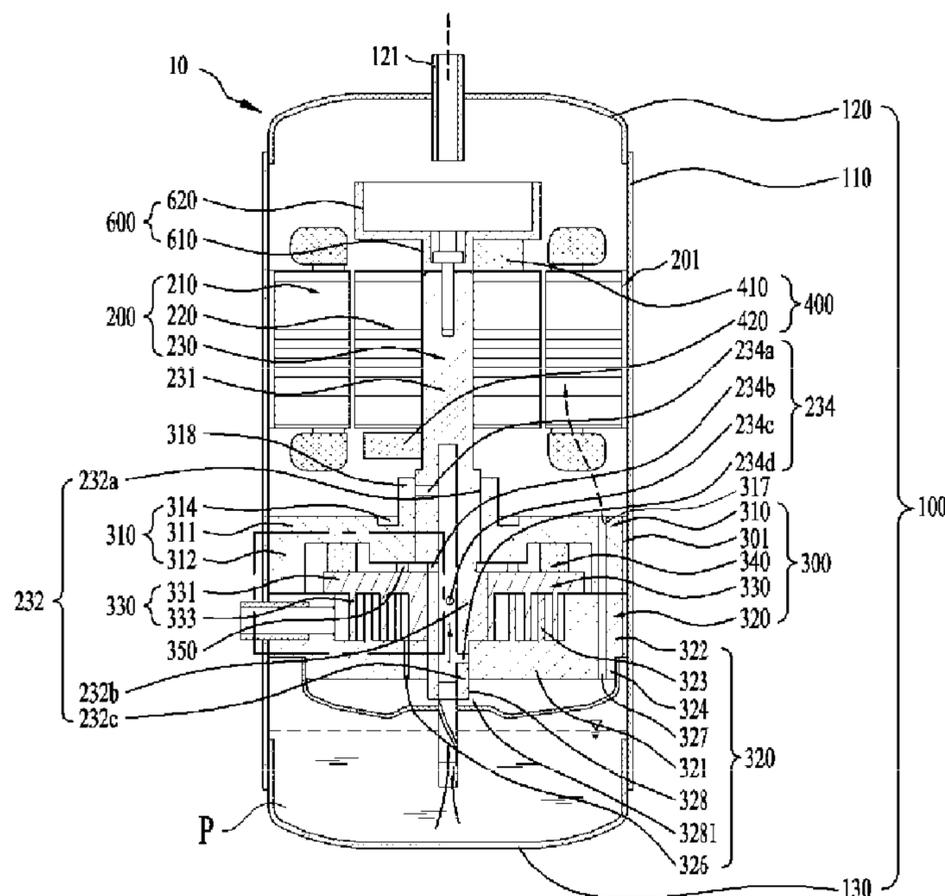
coupler coupled to the rotor or the rotation shaft and configured to rotate the centrifugal separator based on rotation of the rotating shaft.
