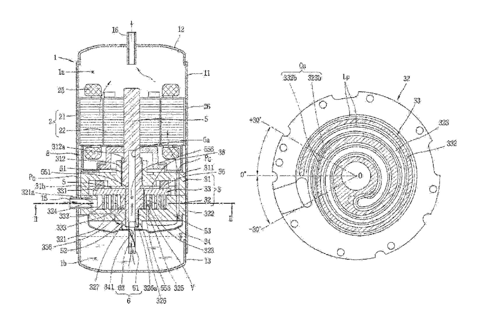
the orbiting wrap at an opposite side to the suction chamber, resulting in enhanced compression efficiency.
