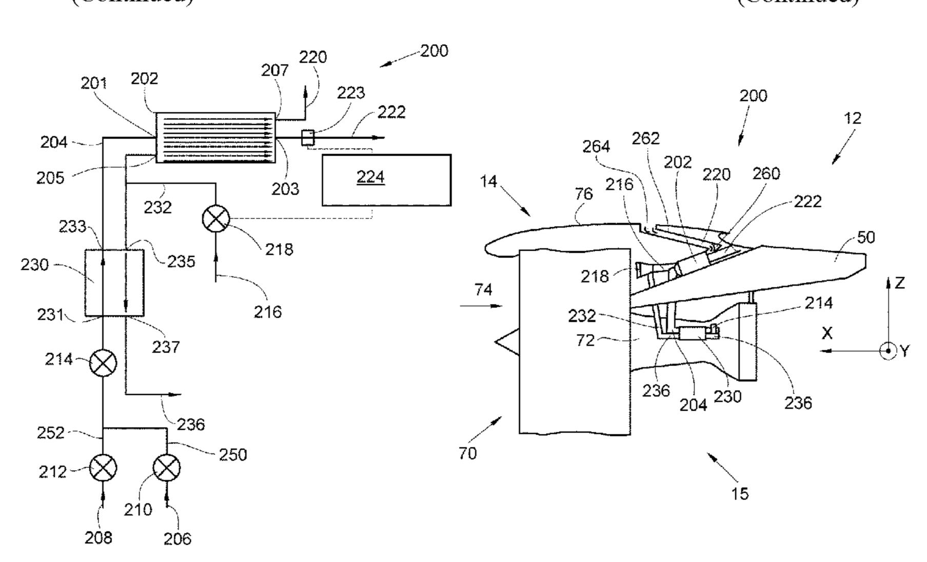
supplying cold air from the main supply pipe, a sub evacuation pipe expelling air to the fan duct, a temperature sensor measuring hot air temperature exiting the main heat exchanger, and a controller controlling the valves according to the measured temperature.
