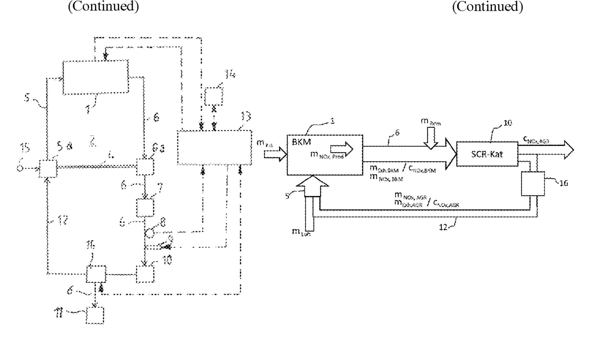
predefined quantity, different from the first quantity; measuring the resulting nitrogen oxide values using the sensor; and determining the efficiency of the SCR catalytic converter based at least in part on the associated exhaust-gas recirculation rate and the measured nitrogen oxide values.
