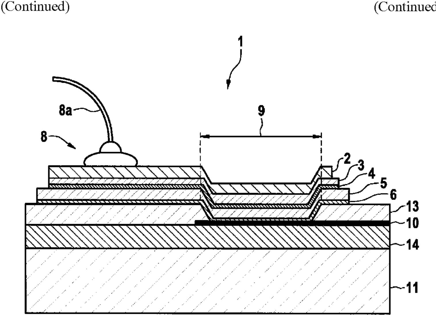
layer. The bonding pad is situated in the area of the contact hole on the semiconductor chip, in which a platinum conductor track leading to the heater is connected using a ring contact and/or is connected outside this area.
