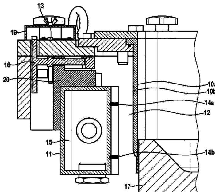
outer side of the running surface (10) and the width of the gap (12) can be adjusted by the adjusting element (13).
