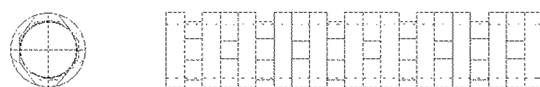
Micro-fabricated catheter shaft with cuts that do not cut through to the lumen.
