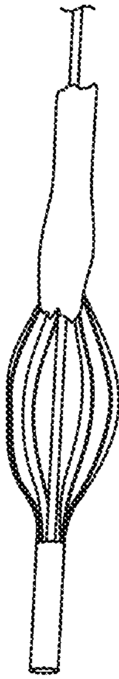
Wide Shape Set and Foam Epoxied Device
