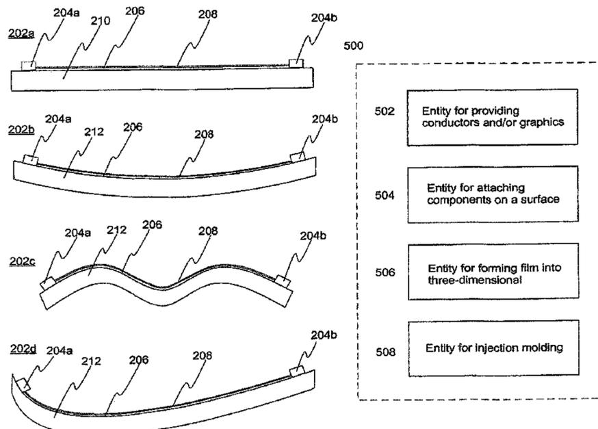
ond, and third entities are arranged relative to one another to manufacture the electromechanical structure.
