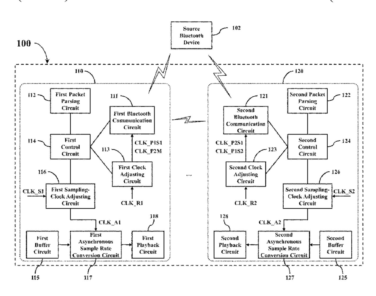
by the source Bluetooth device, and samples a first audio data to be playback. The auxiliary Bluetooth circuit generates a second slave clock and a third slave clock synchronized with the second main clock, and samples a second audio data to be playback.
