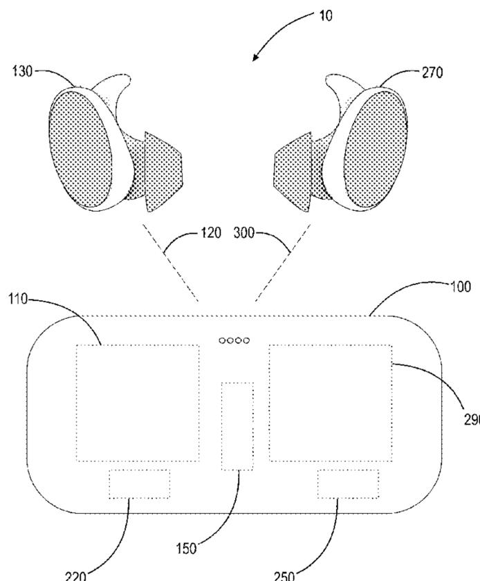
wireless audio device; (2) applying, pre-charge load to the device battery; (3) retrieving the voltage; and (4) transmitting the voltage to the case.
