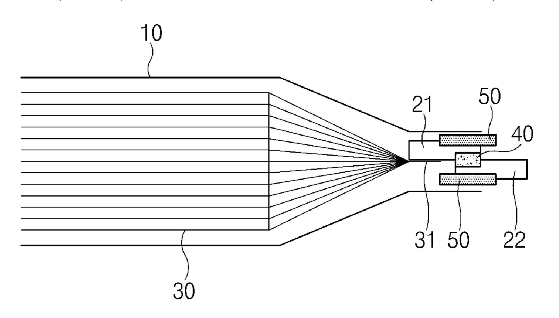
mechanically and electrically coupling the first lead and the second lead to each other; and a high-voltage decomposition material that is configured to generate a gas when a high voltage having a predetermined level or more is applied to the adhesion unit.
