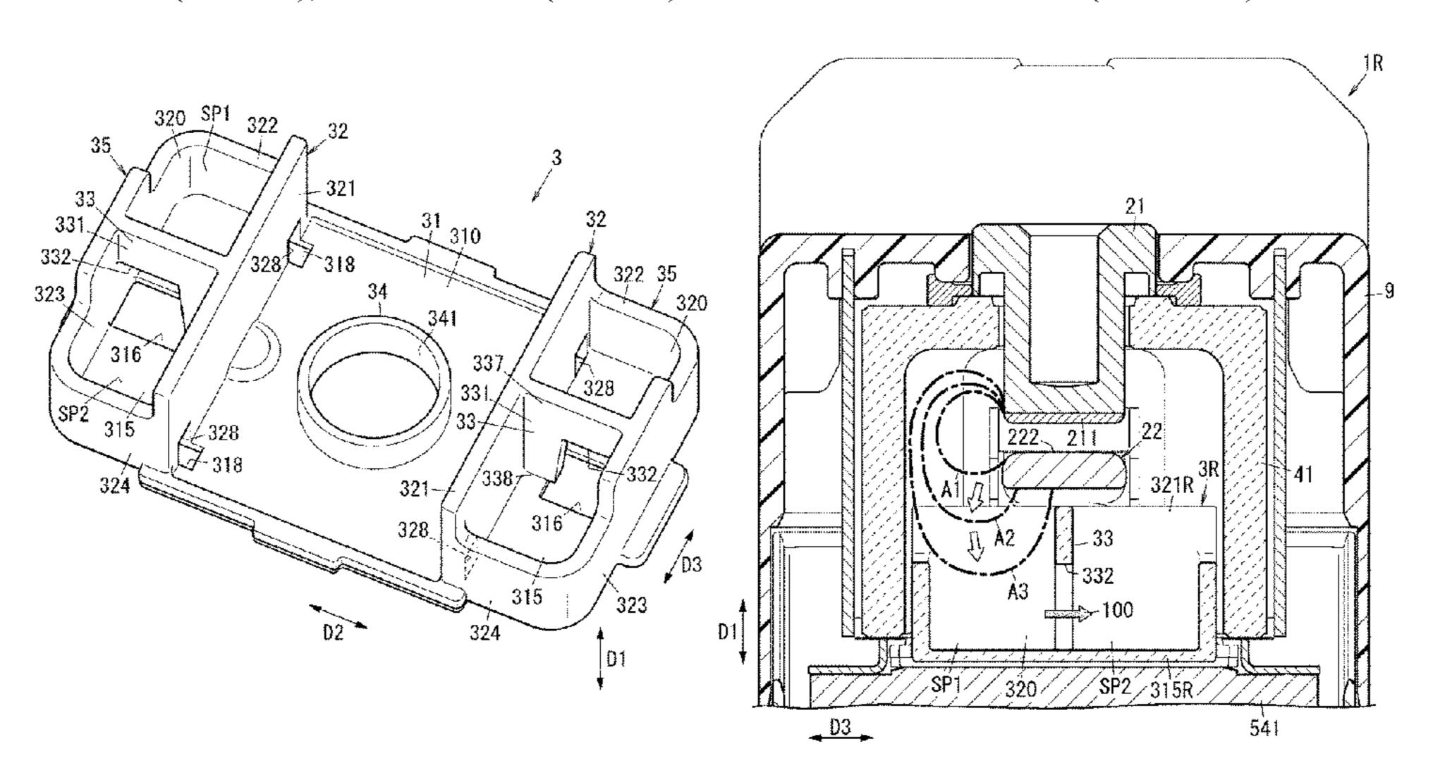
the partition wall is located in the first direction from the fixed contact and the movable contact.
