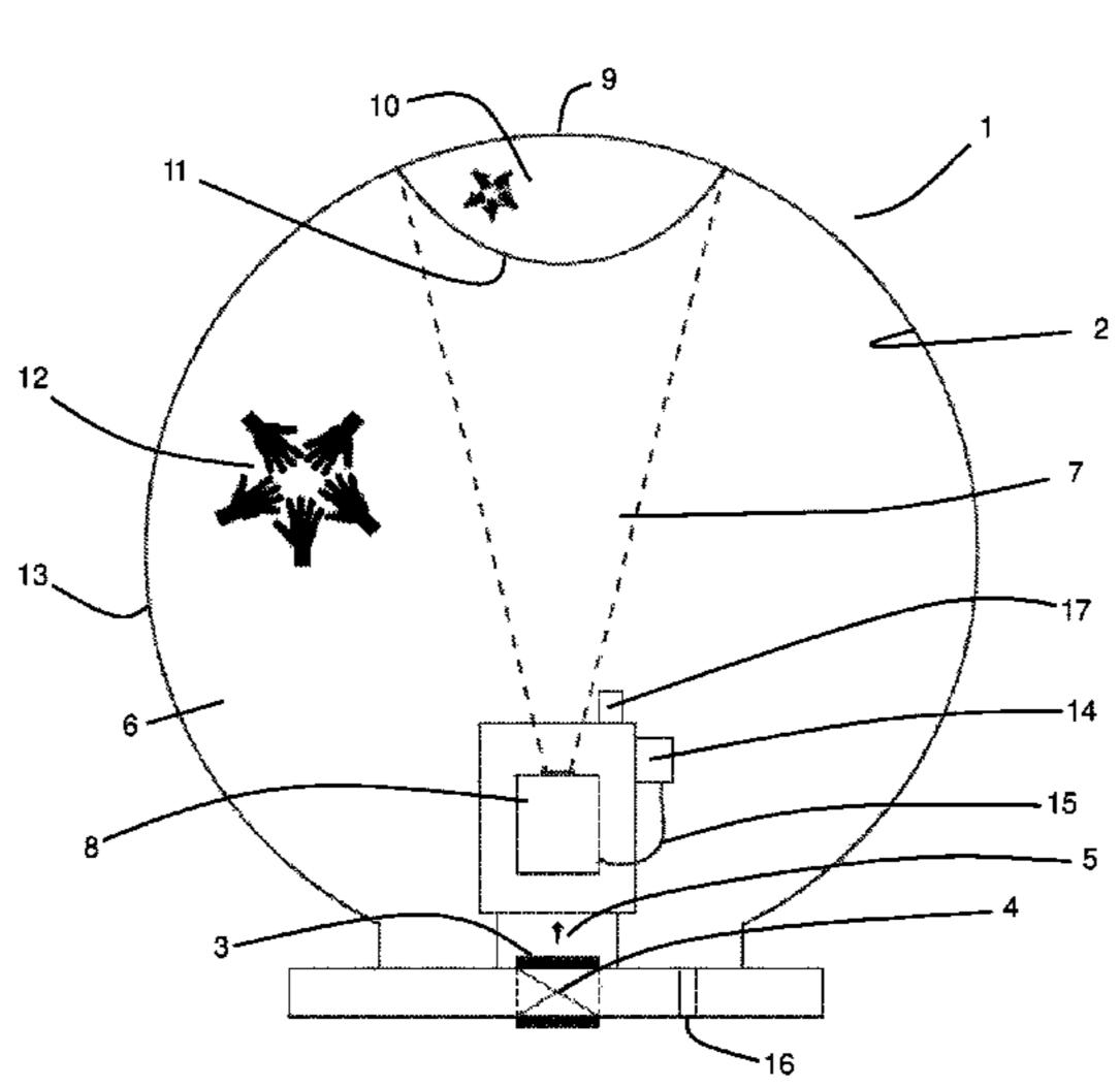
The projector is configured within the interior of the envelope and aligned in such a way that the projector beam is reflected onto the inner surface serving as a three-dimensional projection screen via the reflection mirror.
