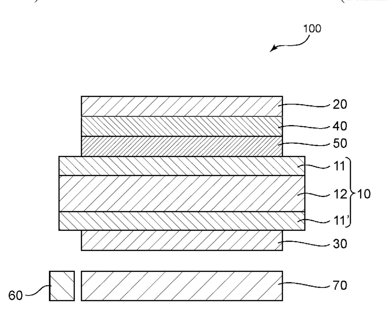
a refractive index  $nz_2$  in a thickness direction of the second optical compensation layer is less than 1.5340.
