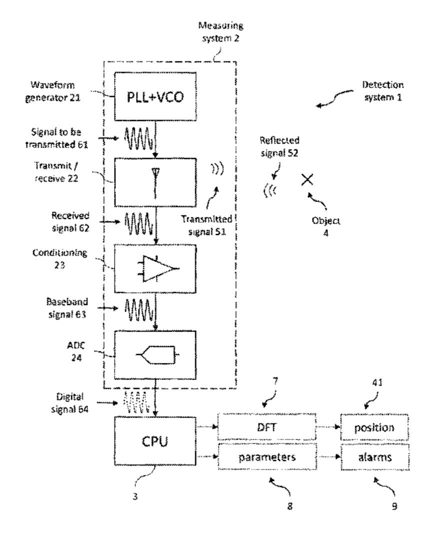
an analog-to-digital converter configured to provide a digital signal which is a discrete sequence of values obtained by sampling the baseband electrical signal in plural time instants.
